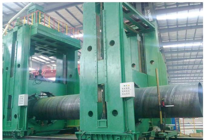
The Lincoln Welder uses an advanced double submerged-arc welding technique
